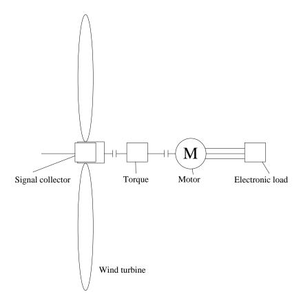
The rotor have 3 blades and diameter is 1.5m The device will be manufactured in next May.
