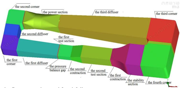
the first test section used for airfoil test:
