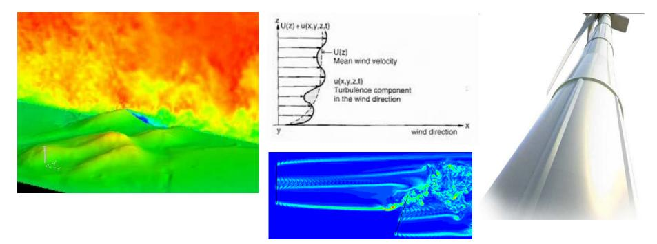
Non-uniform flow filed produces varying loads on blades and structure -> loads amplification and fatigue damage
