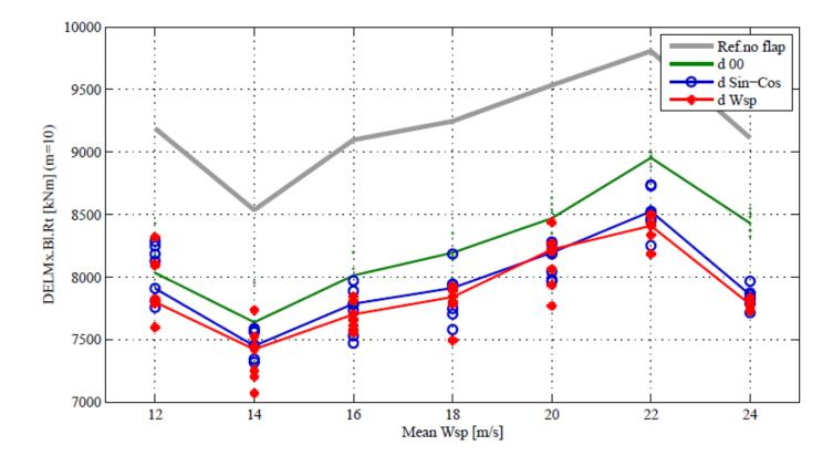
Lifetime fatigue DEL alleviation: (IEC conditions IIb)
