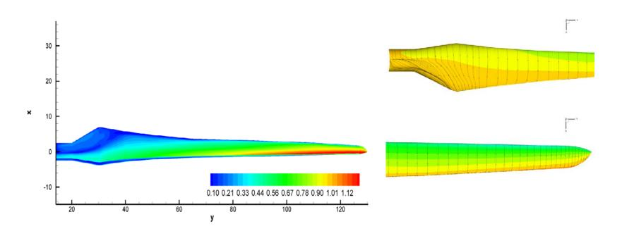
Good agreements are observed between results from BEM and CFD methods. CFD predicts slightly higher forces than BEM which is observed from 40m < r < 130m. Such a difference is often caused by the rotational effect that has been modelled by CFD but not enough counted by BEM.
