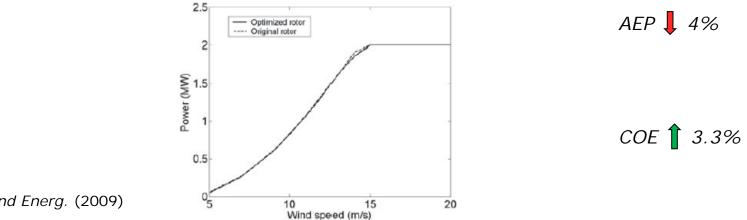
Figure 12. Power performance of the original and the optimized Tjæreborg 2 MW rotor
