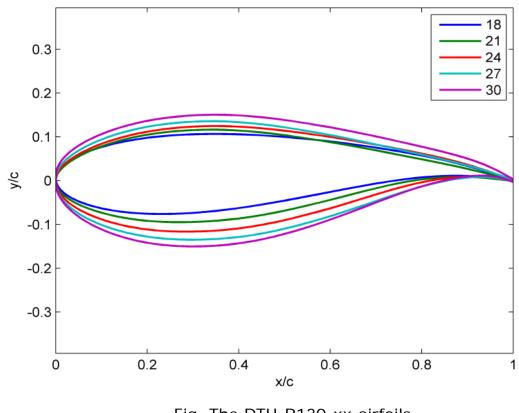
Fig. The DTU-R130-xx airfoils
