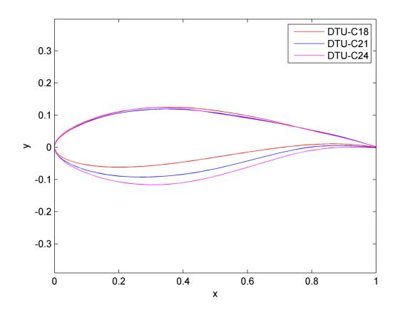
wind tunnel tested for aerodynamics: C18,C21,C24
