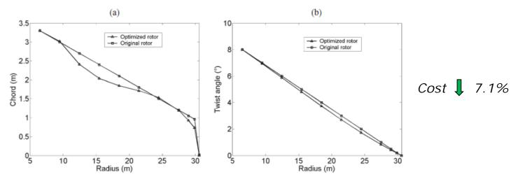
Figure 11. (a) Chord and (b) twist angle distributions of the original and the optimized Tjæreborg 2 MW rotor
